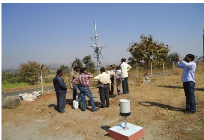
Figure 9-1: Automatic Rainfall Station.
