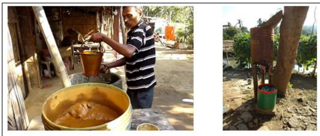
Figure 10-3 Indigenous iron filter system
